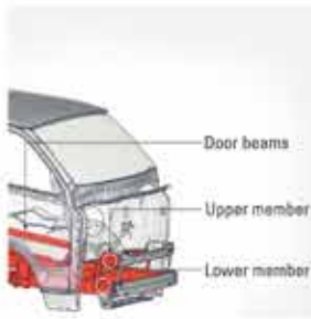
New upper and lower front frame members
