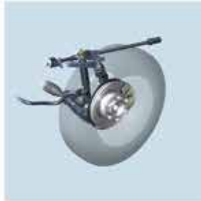
Front suspension - double wishbone
