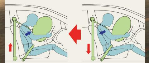
Front Seat Belts: 3-Point ELR with Pretensioner and Force Limiter GOA Body with Reinforcements
