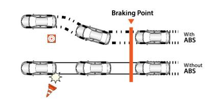
Anti-lock Braking System with Electronic Brake-force Distribution
