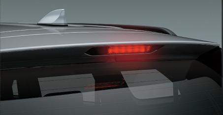
High Mount Stop Lamp with Shark Fin Antenna
